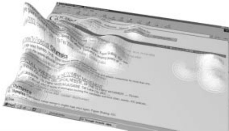
Figure 1.2 Contour map of Google showing the intensity of eye fixations. Higher peaks indicate regions of more fixations (Feusner, 2004).
