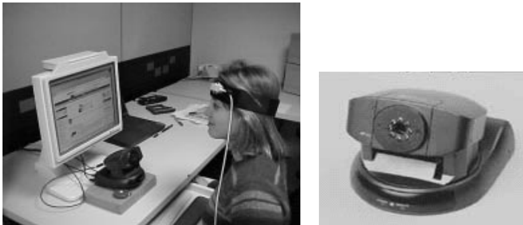
Figure 3.1 Subject with eye tracking apparatus (left); close-up of pan/tilt camera unit.
